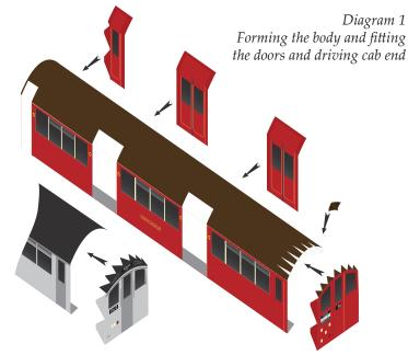
Note the different roof ends. The right hand diagram shows 1935/38 stock the left hand diagram shows the straight end on 1956/59/62 stock
